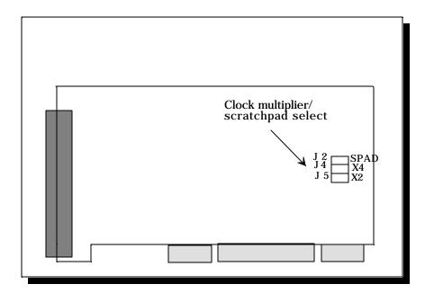
Figure 5 --- Jumper/connector locations
